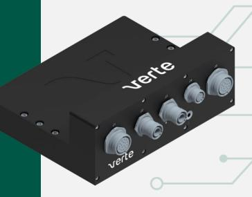
VERTE Elektronik's SSPDU-270D-14-140-BXX series is designed as a high-power density, low-profile power distribution unit. This unit, which has 14 channel outputs, distributes the input voltage in the range of 100-400 V to the loads via semiconductor switches and provides overload and short circuit protection. The device can be controlled and configured via CAN and RS-422/485 communication interfaces, and status information can be displayed.
